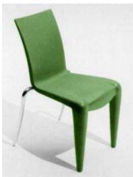
The Louis 20 chair by Philippe Starck is made from only aluminium and polypropylene, both over 99% pure. The chair is held together with only five screws, making it very easy to disassemble and recycle. Source: www.biothinking.com
